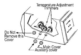
If the unit is not recording the proper temperature, use the following procedures. If the temperature is off by more than 10 degrees of actual there is some other problem with your unit. (Do not attempt to re-calibrate).
