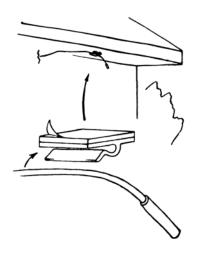
Run the main sensor through a window or any other convenient topening. The ideal location for he sensor is under the eave on the north side of the building.
